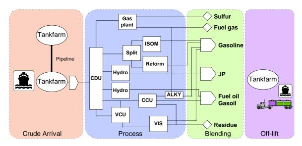
Figure 6: Refinery schematic diagram
