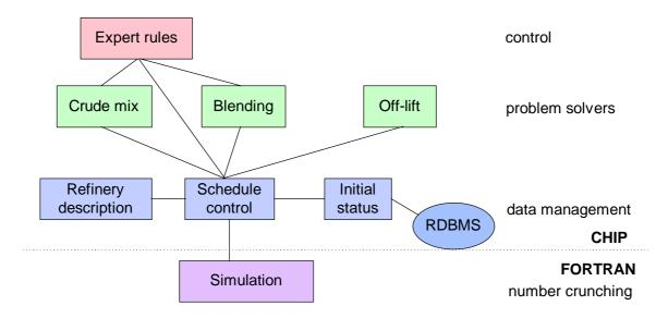
Figure 7: FORWARD system modules
